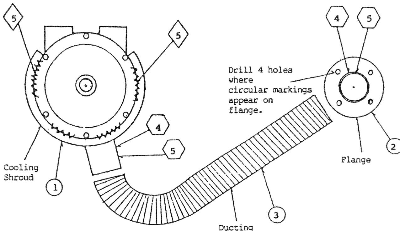
**Note:** Shroud must be centered on the pump. On some installations the pump may have to be rotated on the mounting pad because of interference with other objects.
