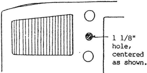
View: L H rear engine baffle,
