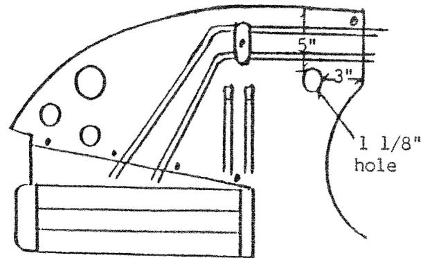
View: L H rear engine baffle, looking forward.
