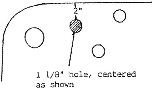
View: L H rear engine baffle,
